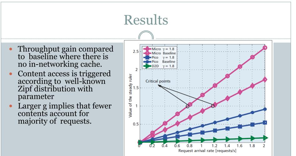
When g = 1.8 throughput gain is 53.9 percent that of baseline. Pico and D2D tiers are far from fully loaded state when micro tier comes to critical steady state.
