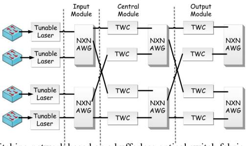
Petabit: full optical switching network based on a bufferless optical switch fabric.
