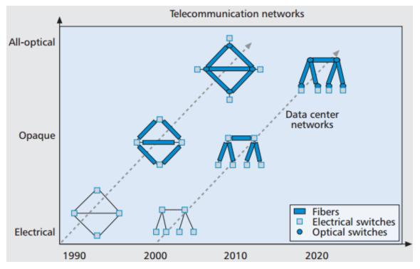
At the telecommunications networks side, opaque networks based on point-topoint optical fibers have recently been replaced by all-optical (transparent) networks.
