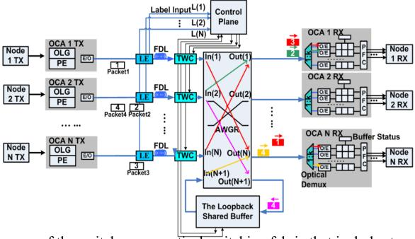
**DOS** contains a core of the switch are an optical switching fabric that includes tunable wavelength converters (TWC), a uniform loss and cyclic frequency (ULCF) AWGR, and a loopback shared buffer system. a control block that processes the label of the packet and then arbitrates each packet by checking resource availability on the output port side.
