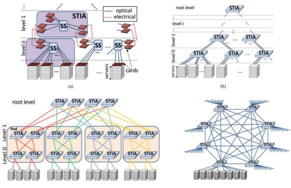
**Space-time interconnection architecture (STIA)** utilizes the space domain to switch packets and the time domain to switch packets to different nodes.
