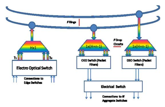
**Fission** DCN architecture comprises fiber rings that are used to interconnect the core data center switches by deploying ultra-dense WDM (UDWDM) technology.
