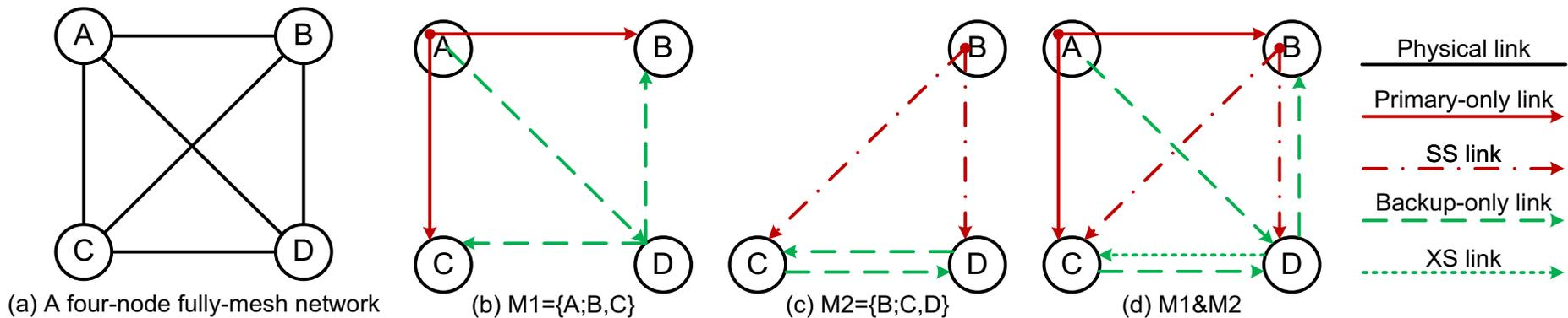
An example for protection schemes: (a) a four-node fully-mesh network; (b) link-disjoint; (c) self-sharing; and (d) cross-sharing.
