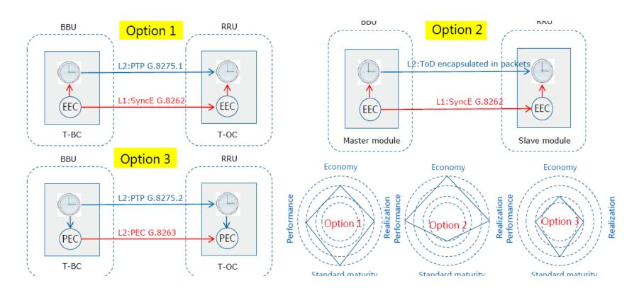
Option 1: T-BC and T-OC are located in BBU and RRU respectively with G.826x and G.827x series standards supporting compatible with packet networks
