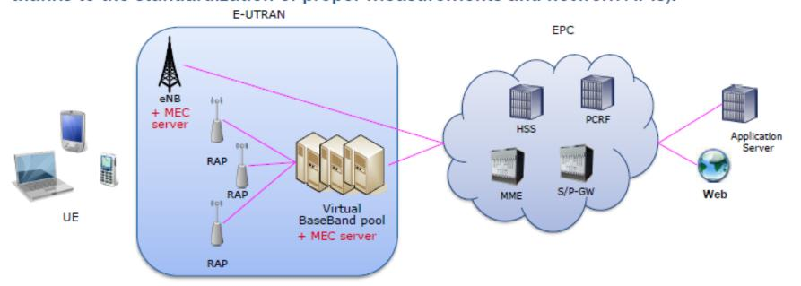
➤ This view is not in contrast with C-RAN architecture: MEC will add flexible decentralization and proper dynamic instantiation of applications, in close proximity to terminals (that are also empowered with additional capabilities through computation offloading).
