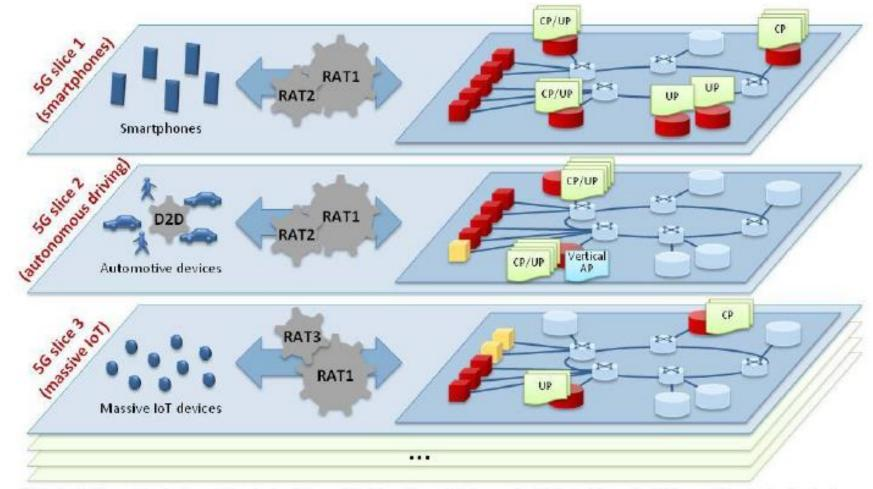
RAT= Radio Access Technology; CP = Control Plane; UP= User Plane; AP= Access Point; IoT= Internet of things; D2D = Device to Device
