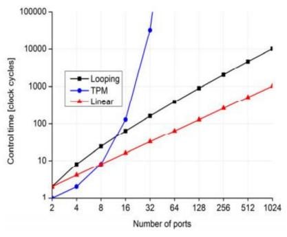
• Configuration time of a Beneš switch expressed in clockcycles according to looping algorithm, Trial Partition Machine [TPM] and an algorithm that scales linearly with the port-count.
