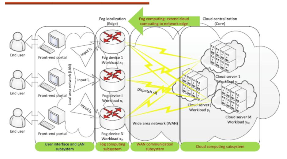
Overall architecture of a fog-cloud computing system with four subsystems and their interconnections/interactions.
