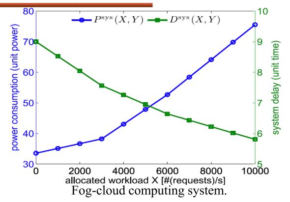
Finally, based on the above  $x_{i}^{*}$  and  $y_{j}^{*}$ , we further solve SP3 and obtain the communication delay  $D^{comm}(X, Y)$  in the WAN subsystem. Based on these we calculate the system power consumption  $P^{sys}(X, Y)$  and delay  $D^{sys}(X, Y)$ . we note that the power consumption of fog devices dominates the system power consumption, while the communication delay of WAN dominates the system delay.
