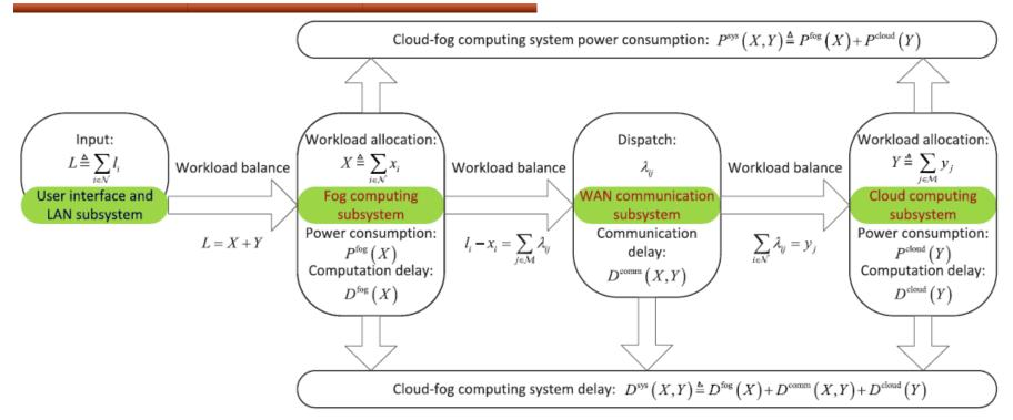
framework of power consumption-delay tradeoff by workload allocation in a fog-cloud computing system
