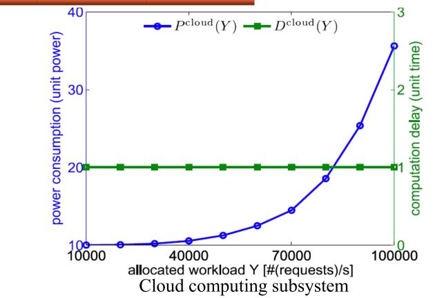
Then, they vary the workload Y allocated for cloud computing from  $10^4$  to  $10^5$ , to evaluate how they affect the power consumption  $P^{cloud}(Y)$  and computation delay  $D^{cloud}(Y)$  in the subsystem. The result shows that the computation delay stays steady while the power consumption increases with the workload allocated for cloud
