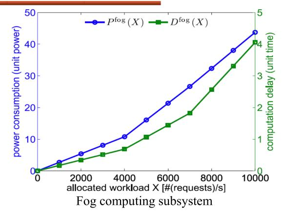
They vary the workload X allocated for fog computing from 0 to  $10^4$ , to evaluate how they affect the power consumption  $P^{fog}(X)$  and computation delay  $D^{fog}(X)$  in the subsystem. It is seen that both power consumption and computation delay increase with the workload allocated for fog computing.
